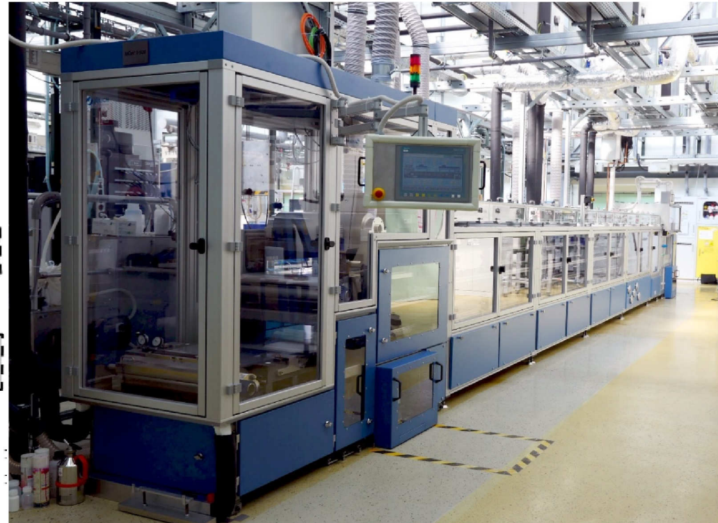
JuCast 3-500: Sequential tape caster with three casting heads
